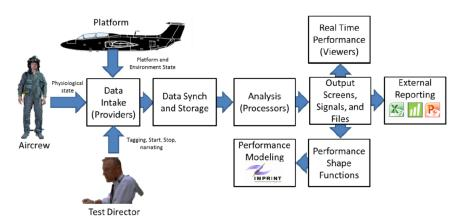
**Analytics Application:** The analytical software and its user interface aggregates, synchronizes, tags, analyzes, and visualizes human and aircraft data in real time.
