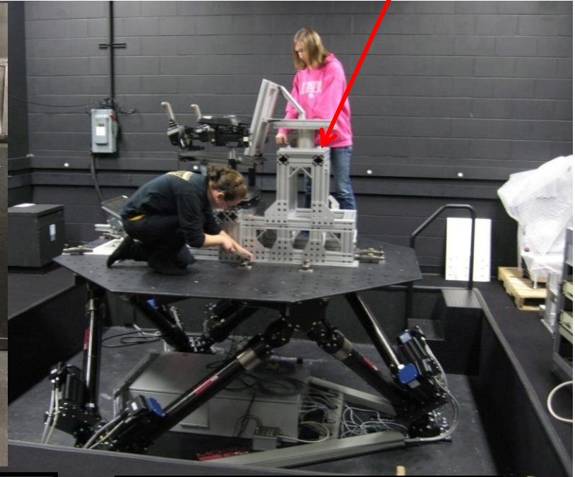
Six-degree of freedom Moog FCS motion platform
