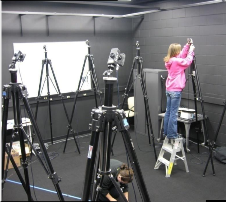
12 cameras Vicon motion tracking system
